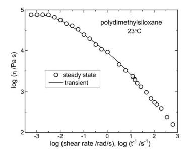
**Figure 27.** Viscosities determined from steady state (symbols) and the transient (eqn (5.46); line) shear stress measurements on a branched PDMS ( $M_w = 4.7 \times 10^5$  g/mol). Data from ref. [118].
