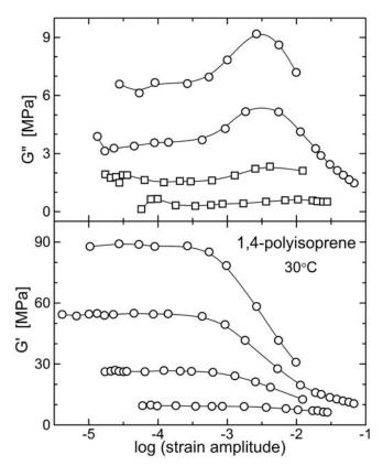
**Figure 29.** Dynamic storage (lower) and loss modulus (upper) versus strain for PI at 0.1 Hz and 30°C. At low strains the modulus is constant, with higher amplitudes disrupting the filler network. Data from ref. [149].
