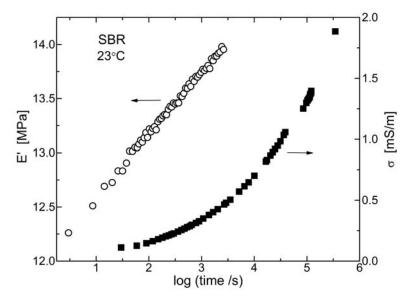
**Figure 30.** Low strain storage modulus (open circles) measured at 40 Hz for an SBR network with 82.5 phr N339 carbon black and 62.5 phr oil, following a static strain of 1.9%; the corresponding DC-conductivity (filled squares) is also shown. The values of E' (= 15.0 MPa) and  $\sigma_{DC}$  (= 4.2×10<sup>-3</sup> S/m) prior to the static strain are substantially larger than attained after recovery (which extended to four days for the electrical measurement).
