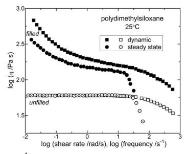
**Figure 22.** Comparison of  $\eta^*(\omega)$  (squares) and  $\eta(\dot{\gamma})$  (circles) for neat PDMS (open symbols) and hydroxylterminated PDMS containing 12.9% by volume calcium carbonate (solid symbols) ( $M_w = 1.3 \times 10^5$  g/mol). Only the former conforms to the Cox-Merz rule. The steep decrease in the steady state viscosity at shear rates > 20 rad/s is due to flow instabilities as the test specimen begins to fracture. Data from ref. [110].
