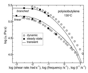
**Figure 26.** Viscosities determined from dynamic (open circles), steady state (solid squares), and the transient (eqn (5.46); line) shear stress measurements on a linear ( $M_w = 5.0 \times 10^5$  g/mol) and a highly branched ( $M_w = 1.08 \times 10^6$  g/mol) PIB. Data from ref. [107].
