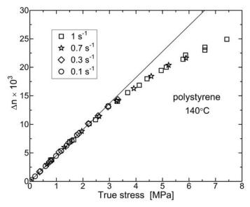
**Figure 8.** Birefringence *versus* true stress for a PS melt (Mw = 206 kg/mol) during uniaxial extension at the indicated strain rates. The data superpose with deviation from the stress optic law observed for  $\hat{\sigma} > 2.2$  MPa. Data from ref. [33].
