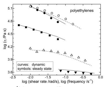
**Figure 21.** Comparison of  $\eta^*(\omega)$  (symbols) and  $\eta(\dot{\gamma})$  (lines) for high density polyethylenes (HDPE, composed of primarily linear chains; solid symbols;) and low density polyethylenes (LDPE, which has branching on about 2% of its carbon atoms; open symbols). Different symbols correspond to different  $M_w$ , in the range from 100 – 140 kg/mol with substantial polydispersities ( $\geq 4$ ). Temperature for HDPE is 190°C and for LDPE = 175°C. Data from ref. [103].
