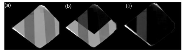
**Figure 5.** (a) Natural rubber double network (on left) and conventional NR elastomer (on right), both in a state of mechanical equilibrium ( $\sigma = 0$ ); nevertheless, (b and c), through crossed polarizers the double network transmits light, due to its inherent orientation. Since the external stress is zero, this is a violation of the stress optic law, eqn (5.14).
