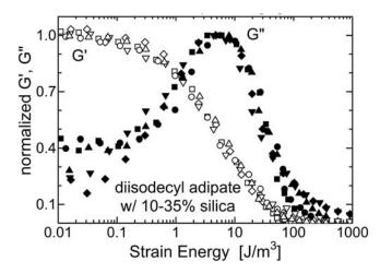
**Figure 32.** (upper) Dynamic storage (open symbols) and loss (filled symbols) moduli at 30°C and 0.5 Hz *versus* strain amplitude for the diisodecyl adipate containing 0.10 (squares), 0.14 (circles), 0.20 (triangles), 0.30 (down triangles), and 0.35 (diamonds) volume fraction silica particles Data from ref. [164]. (lower) Same data with the storage modulus normalized by the low strain plateau value and the loss modulus by the maximum in G". Data from ref. [163].
