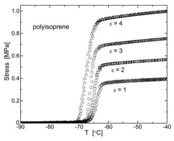
Figure 4. Stress measured in a crosslinked 1,4-polyisoprene during heating at 1 K/min. The sample was initially stretched at RT to the indicated tensile strain and then quenched below  $T_g$ . Data from ref. [25].
