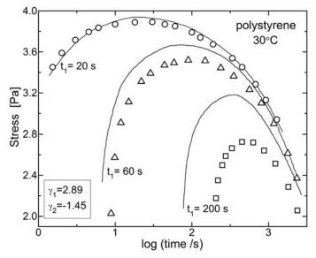
**Figure 15.** Shear stress for polystyrene ( $M_w = 670 \text{ kg/mol}$ ) solution for shear strain = 2.89 imposed at t = 0 and reduced to 1.44 after the indicated time intervals. Equation (5.5) (solid curves) increasingly over-estimates the stresses with increasing time between successive steps. Data from ref. [84].
