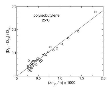
**Figure 9.** Normalized difference in thermal diffusivity *versus* normalized birefringence for polyisobutylene ( $M_w$  = 85 kg/mol) after a step shear strain equal to eight. The solid line through the data suggests a proportionality between these quantities. Data from ref. [36].
