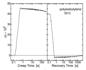
**Figure 20.** Strain and birefringence for PIB ( $M_v = 9 \times 10^5$  g/mol). Data below *ca.* 1 s reflect the instrumental rise time. The decrease in  $\Delta n$  during creep is caused by the reduction in stress due to the changing cross-sectional area; the stress-optical coefficient actually increases slightly with strain. The birefringence has an opposite sign during the stress-free recovery. Data from ref. [91].
