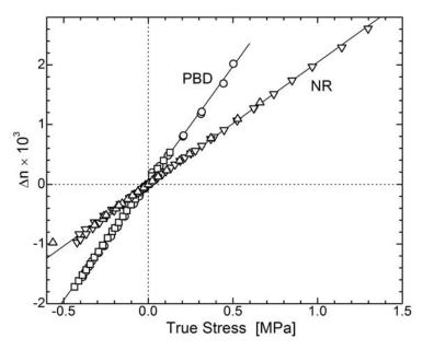
**Figure 6.** Birefringence as a function of true stress for the cross-linked 1,4-polybutadiene and natural rubber subjected to tension and compression; the slopes yield 3.6 and 2.0  $\text{GPa}^{-1}$  for the respective stress optical coefficients. Different symbols represent different test specimens. Data from ref. [27].
