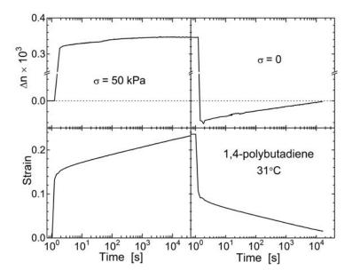
**Figure 19.** Shear strain and associated birefringence of cross-linked PBD during creep and recovery. The birefringence becomes measurably invariant at  $10^4$  s, although the compliance never reaches steady state. The sign of  $\Delta n$  changes upon removal of the load. Data from ref. [27].
