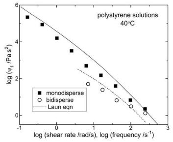
**Figure 24.** Experimental (symbols) and calculated (eqn (5.40); solid and dashed lines) first normal stress coefficient for monodisperse ( $M_w = 2 \times 10^6$  g/mol; P = 1.09) and bidisperse ( $M_w = 7 \times 10^5$  g/mol blended with 8%  $M_w = 2 \times 10^6$  g/mol) polystyrene 20% solutions. Data from ref. [112].
