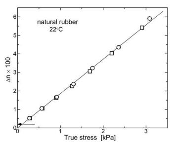
**Figure 18.** Birefringence from uncrosslinked NR under uniaxial tension. Measurements were made upon increment of the stress and after some subsequent creep. The arrow indicates the magnitude of  $\Delta n$  measured about 2 min after removal of all stress. Data from ref. [90].
