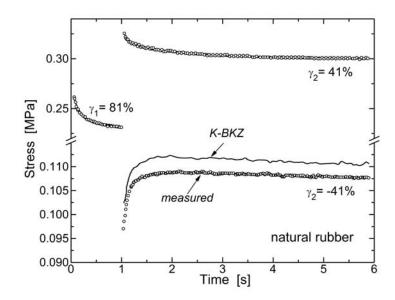
Figure 14. Stress measured for cross-linked NR subjected to double-step shear strains (circles) of the indicated magnitudes and sign. The second step was applied at  $t_1 = 1$  s after the initial strain. The stresses calculated from eqn (5.38) for  $t > t_1$  (solid line) are only evident for the reversing strain history ( $\gamma_2 + \gamma_1 < \gamma_1$ ; lower curves), being masked by the experimental points for the stress-increasing deformation. Data from ref. [80]
