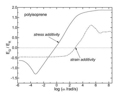
**Figure 12.** The relative contribution of the distortional and orientational components of the stress birefringence, as reflected in the magnitude of the respective glassy and rubbery moduli, determined from the data in **Figure 43** using eqn (5.25) (solid line) or eqn (5.34) (broken line). The horizontal dotted line denotes equal contribution from the two components.
