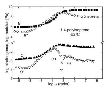
**Figure 11.** Time-temperature master curves of the dynamic moduli (upper curves) and strain optical coefficients (lower curves) for PI. There is a change in sign of  $O''(\omega)$  at log  $\omega = 2.5$ . Data from refs. [39].
