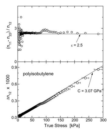
**Figure 7.** (bottom) Birefringence *versus* shear stress for uncrosslinked PIB following a step shear strain = 2.5. Solid curve is the linear fitting yielding the indicated stress optical coefficient. (top) Ratio of refractive index components (1 is the flow direction and 2 the direction of the gradient). is constant and equal to the shear strain, in accord with eqn (5.8). Data from ref. [30].
