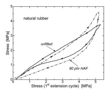
**Figure 13.** Engineering stress for networks of gum NR and NR with carbon black during the  $2^{nd}$  cycle of extension-retraction *versus* the stress for the initial extension. The strain rate was 0.03 s<sup>-1</sup>. Data from ref. [77].
