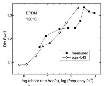
**Figure 25.** Experimentally measured  $\hat{D}$  (solid square) for carbon black reinforced EPDM compound sheared in a capillary rheometer, along with the values (open circles) calculated from dynamic measurements using eqns. (5.40) and (5.44). Data from ref. [116].
