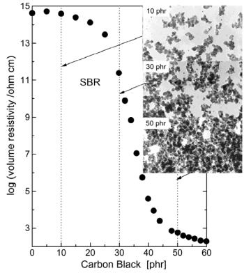
**Figure 28.** Transmission electron micrograph images of SBR containing the indicated quantity of N330 carbon black. The corresponding electrical resistivity behavior is indicated in the graph. Data from ref. [147].
